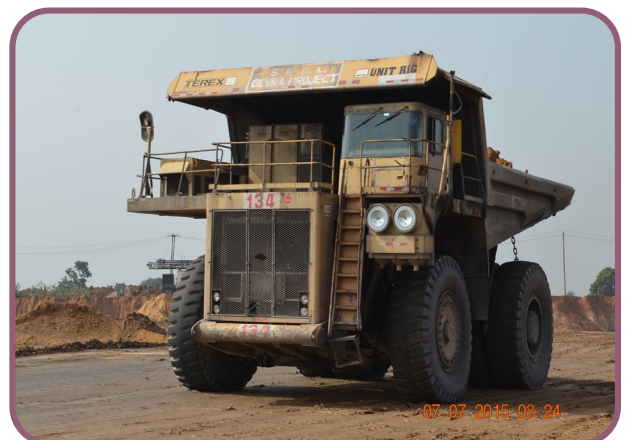
240T Dumper in Operation at Gevra OC
