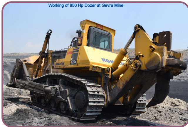
850 HP Dozer in Operation at Gevra OC
