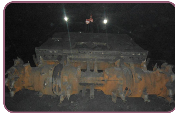
Continuous Miner at Vindhya UG, Johilla Area
