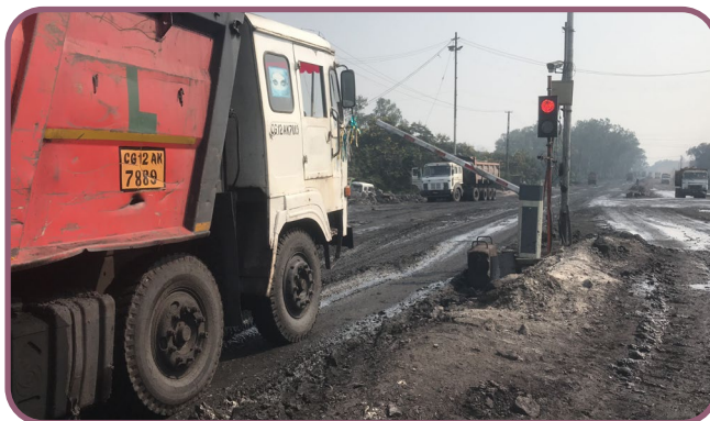
Vehicle waiting at Barrier while sensing RFID tag of authorized vehicle (Red Light)
