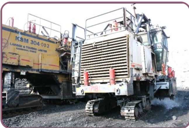
Surface Miner with inbuilt water spraying system
