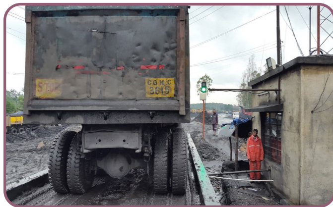
Green light indicates correct position of vehicles at WB during weighing.
