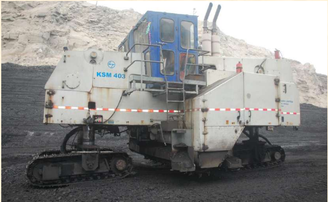
Fig. 14 - Continuous Miner in Operation at Gevra OCP, SECL
