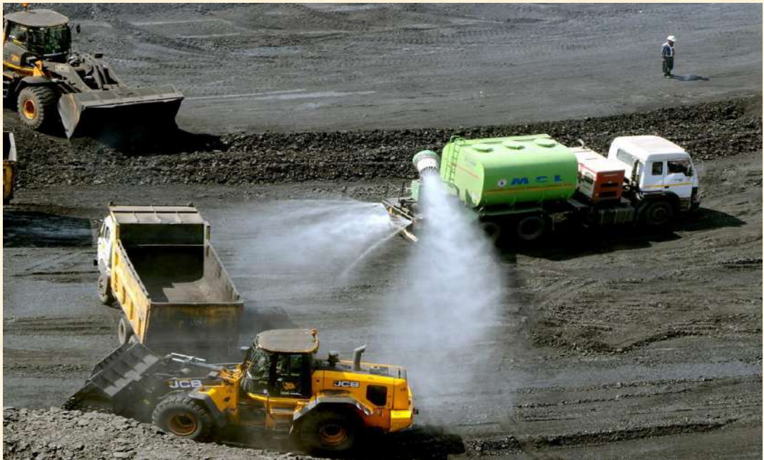
Fig. 47 - Fog Canon in operation for suppression of dust at the source
