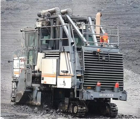
Fig. 28 - Surface miner in operation at SOCP, MCL
