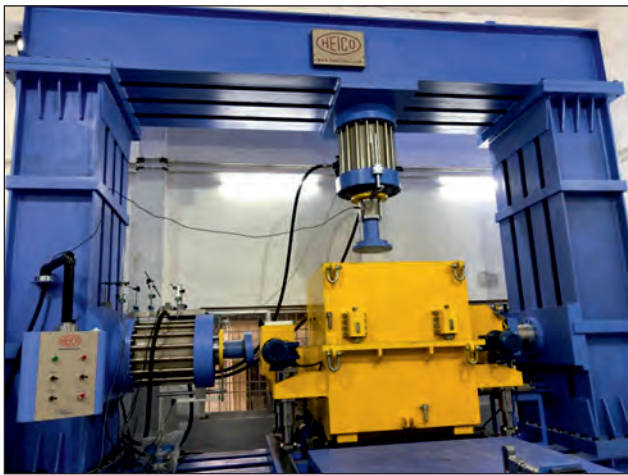
Installation of Large Shear Box Test Machine of 2500 kN capacity (Normal & Shear load)
