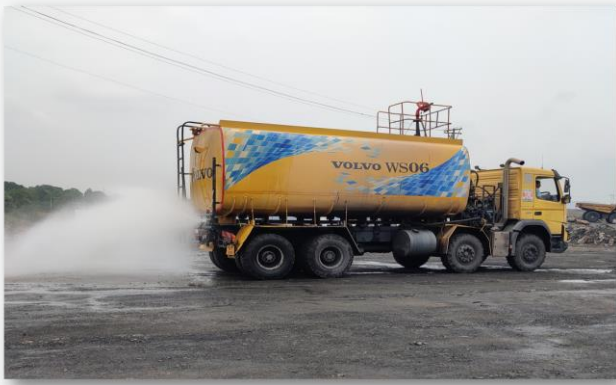
Fig. - Mobile Sprinklers in operation for suppression of dust
