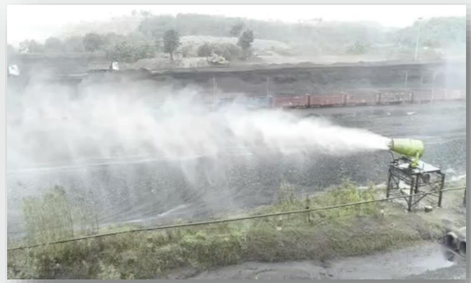
Fig. - Fixed Fog Canon in operation for suppression of dust at the source
